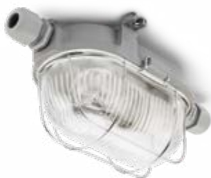
Basement lamp THPG cast iron oval small Length 170 mm, width 125 mm, height 115 mm. Weight 1300 g. Porcelain socket E27, max. 60 W. IP54. Product code 100503
