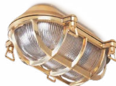
Basement lamp brass large Length 230 mm, width 160 mm, height 110 mm. Weight 1800 g. Porcelain socket E27, max. 60 W. IP54. Product code 130749
