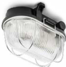
Basement lamp THPG Bakelite oval large Length 195 mm, width 135 mm, height 115 mm. Weight 700 g. Porcelain socket E27, max. 100 W. IP54. Product code 100501
