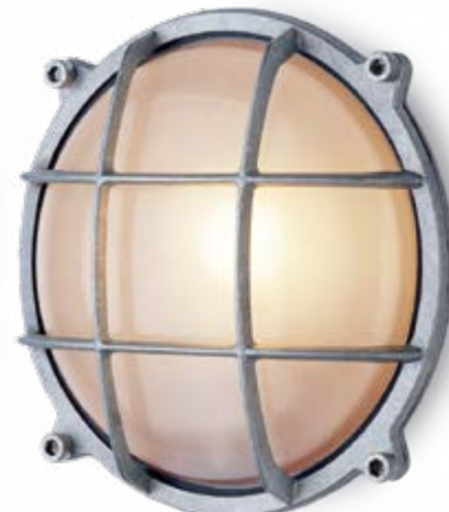
Basement lamp brass large Length 230 mm, width 160 mm, height 110 mm. Weight 1800 g. Porcelain socket E27, max. 60 W. IP54. Product code 130749
