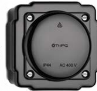
Junction box moisture-proof THPG AC 400 V. For cables up to 4 x 2.5 mm. 95 x 95 x 45 mm. Weight 140 g. IP44.
