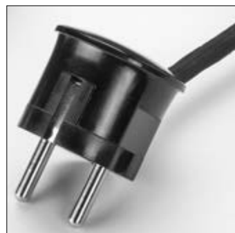
Angled earthing contact plug Duroplast black Black Duroplast. 250 V, 16 A, 50 Hz. Only suitable for alternating current. Length 52 mm. Weight 46 g. Product code 100870
