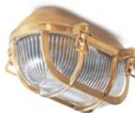
Basement lamp brass large Length 230 mm, width 160 mm, height 110 mm. Weight 1800 g. Porcelain socket E27, max. 60 W. IP54. Product code 130749
