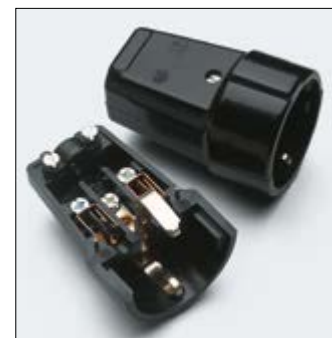
Earthing contact connector Duroplast black Black Duroplast. 250 V, 16 A, 50 Hz. Only suitable for alternating current. Ø 50 mm. Length 70 mm. Weight 68 g. Product code 139448
